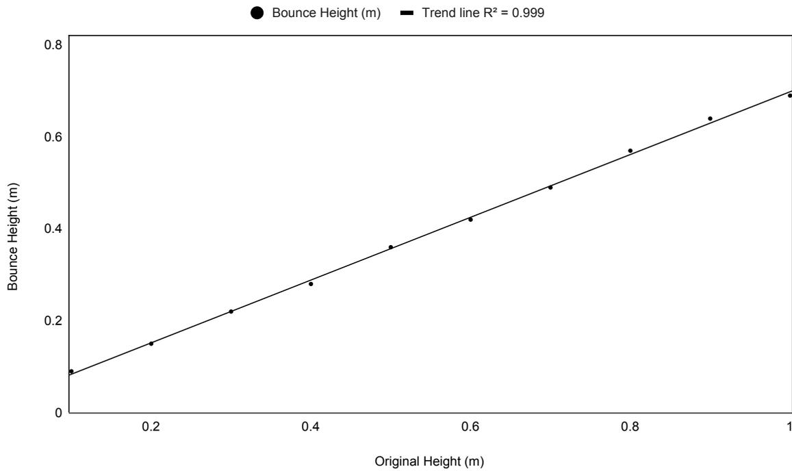
Figure 3.2: Bounce Height vs Original Height Graph (Bouncy Ball 2)
