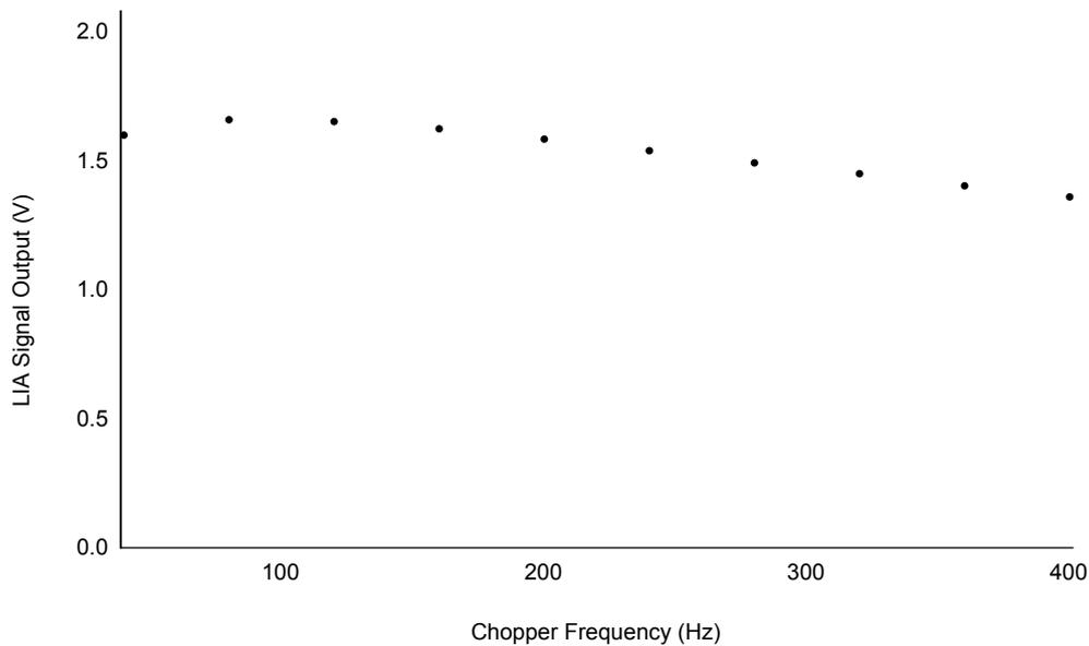
Figure 7: Graph of LIA Signal Output (V) as a function of Chopper Frequency (Hz)
