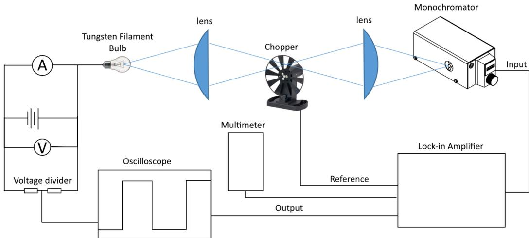
Figure 1: Diagram of experimental set-up for Black-body Radiation Experiment
