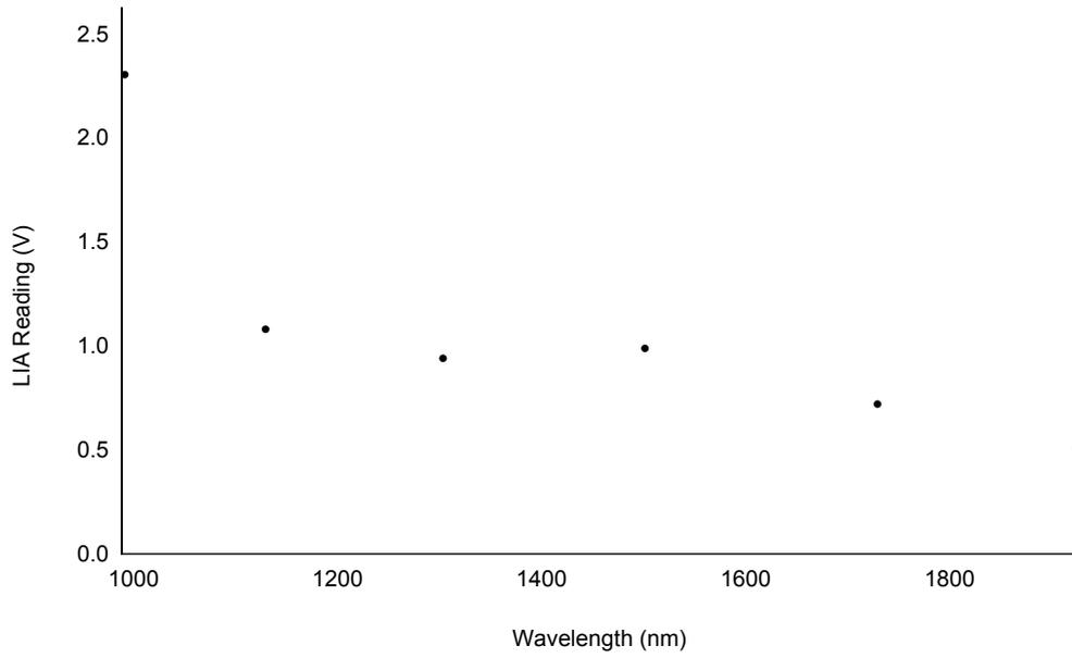
Figure 5: Graph of LIA Reading as a function of Wavelength. (7.5V)
