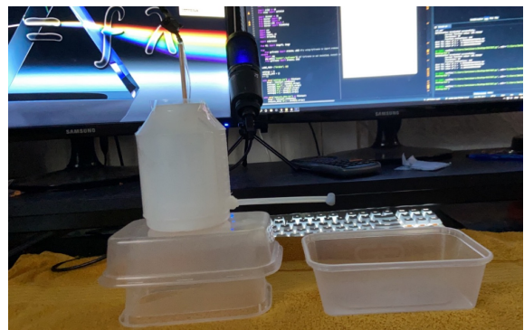
Figure 4: Apparatus with hot glue & supported drain tube
