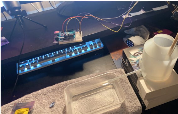
Figure 3: Apparatus with para-film & unsupported drain pipe
