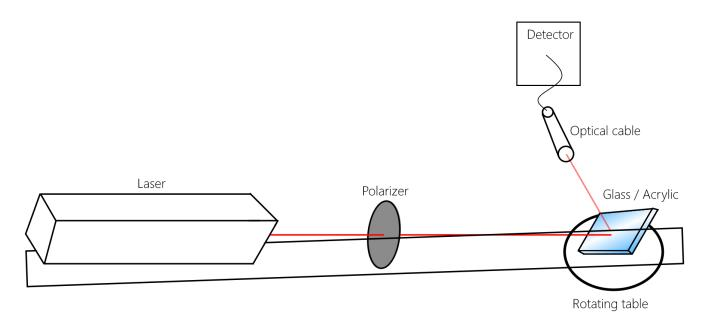
Figure 1: sketch of brewster's angle experimental arrangement
