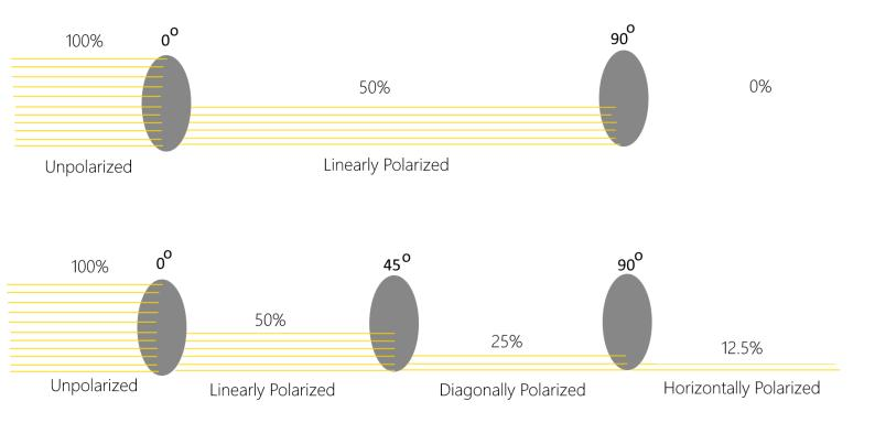
Figure 3: Digram of Triple Polarizer Paradox
