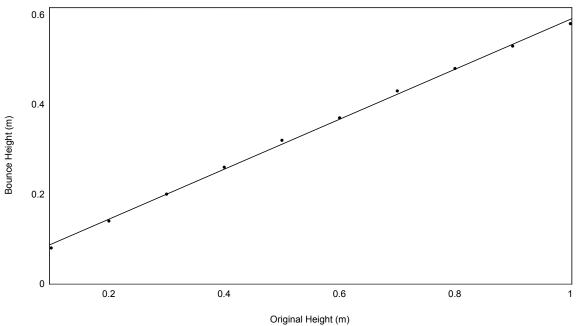
Figure 3.1: Bounce Height vs Original Height Graph (Bouncy Ball 1)
