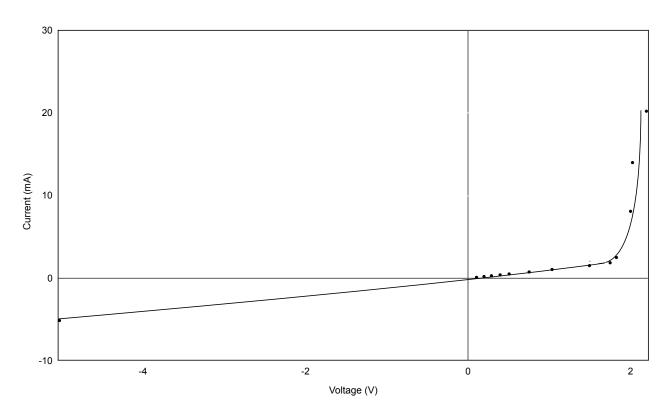
Figure 3.4: Green LED Voltage vs Current
