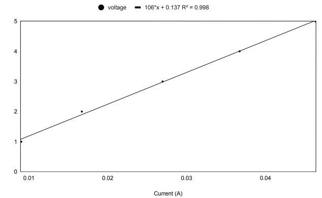
Figure 3.1: Current vs Voltage  $(100\Omega)$
