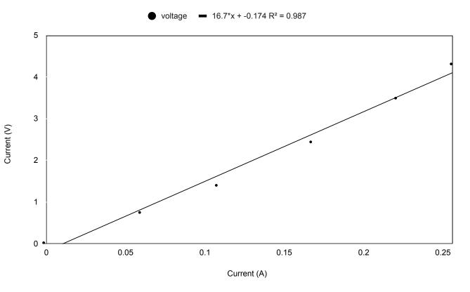
Figure 3.2: Current vs Voltage  $(13\Omega)$
