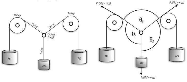
Figure 1.1: Apparatus Diagram Figure 1.2
